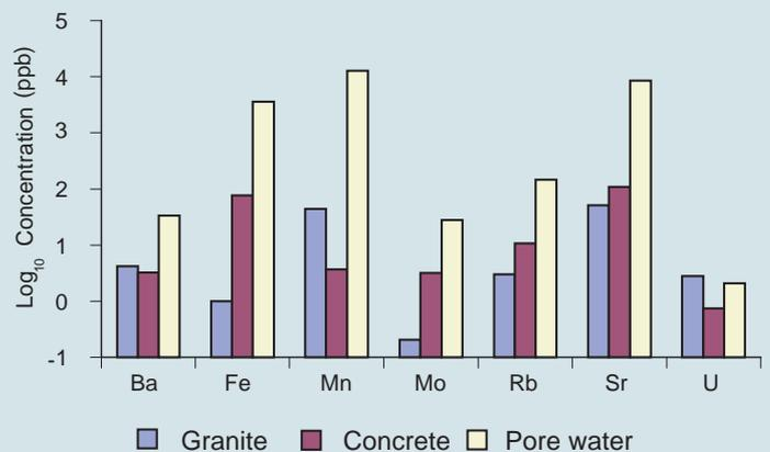
**Fig. 38** A comparison of heavy metal levels derived from granite, sea loch sediment pore waters and the concrete blocks intended for deployment in the experimental artificial reef.
