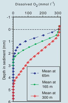
Fig. 3 Interstitial dissolved oxygen profiles from the Beryl "A" cuttings pile showing an increase in oxygen penetration with distance from the platform. The dashed line at 0-mm depth marks the position of the sediment-water interface.
