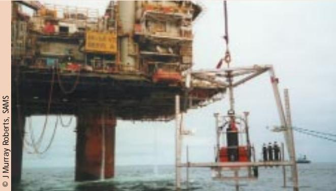
Fig. 51 DML lander being deployed adjacent to the Beryl Alpha production platform
